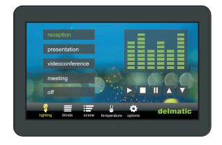
The **touchpanel** is fully software configurable and can include custom graphics and logos, multiple function sub-menus as well as configuration options and user preferences.
